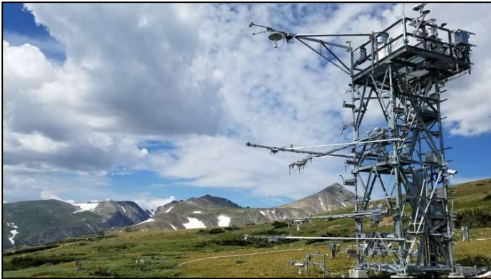
Figure 4. The NEON carbon flux tower located on Niwot Ridge. This structure is about 1000 yards from the LTER station, but measures carbon inputs and outputs from a different area of tundra. Photo from https://www.neonscience.org/field-sites/field-sites-map/NIWO
